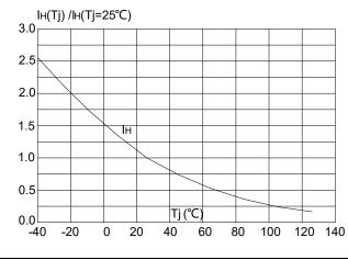
**FIG.4:** On-state characteristics (maximum values)
